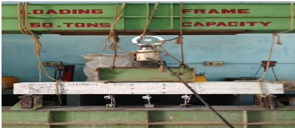
FIG 6: SET-UP OF TEST BEAM IN LOADING FRAME
